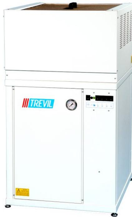
Electric steam generators with 58 litres boiler and modular heating elements. Available from 45 kW to 75 kW size.
